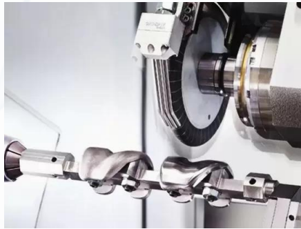
Knee Implant Grinding - Vitrified cBN Wheel
