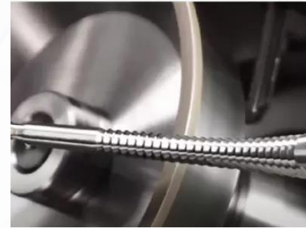
Rasp Grinding - Electroplated Wheel
